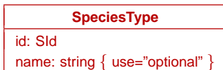
Figure 11: The definition of SpeciesType . Following UML notation, additional fields that are inherited from a base class, in this case Sbase , are not shown.
